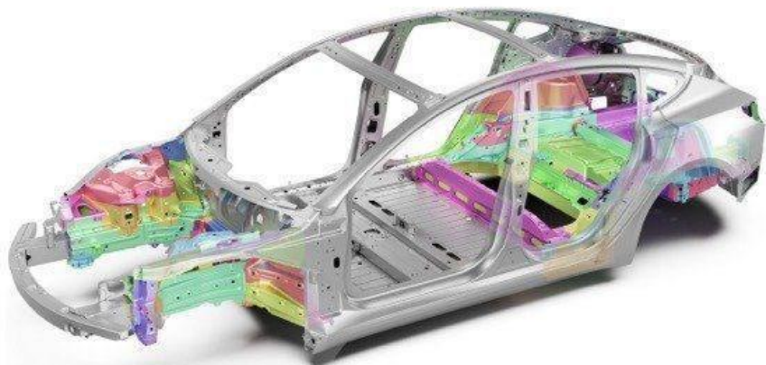
Model 3 body structure 171 pieces of metal highlighted
