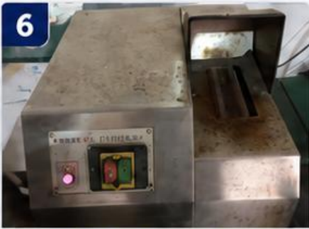
Belt Grinding Machine Reliable grinding for sample surface finishing
