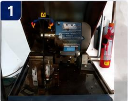
Cutting Machine Precision cutting for sample preparation
