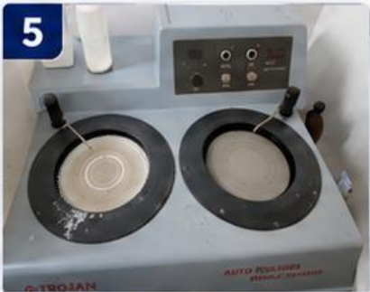
Polishing Machine Mirror-like surface preparation for precise analysis
